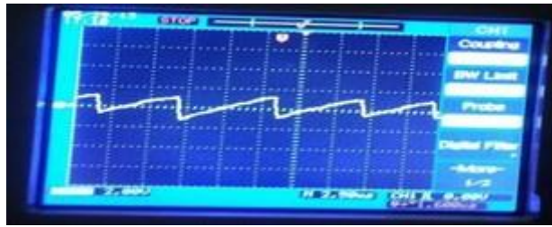
Figure (4.8): Output wave at speaker terminal when noise is high Time scale 2.5 \mu S, Voltage per division 2 V/Div.
