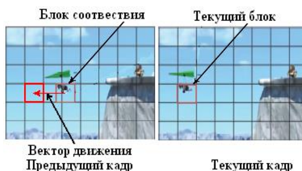
Pic. 1. General principle of block estimation and CD of video objects in adjacent frames.
