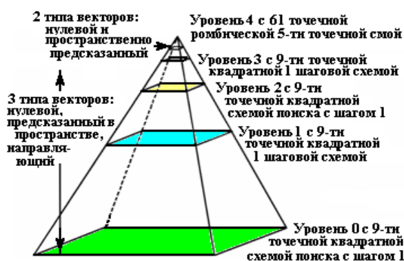
Pic.15. 4-level motion estimation for the CIF format in the Dirac video codec.
