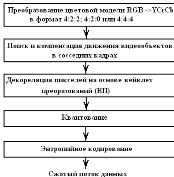
Pic. 5. Main stages of video data processing in the Dirac video encoder.
