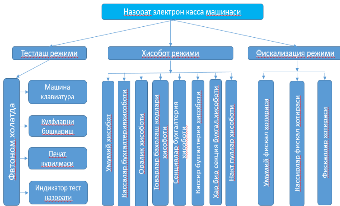
Figure -1. Operation of the control electronic cash register machine in different modes.
