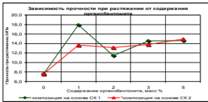
Fig.4. Dependence of tensile strength in the longitudinal direction on the OB content in the composition
