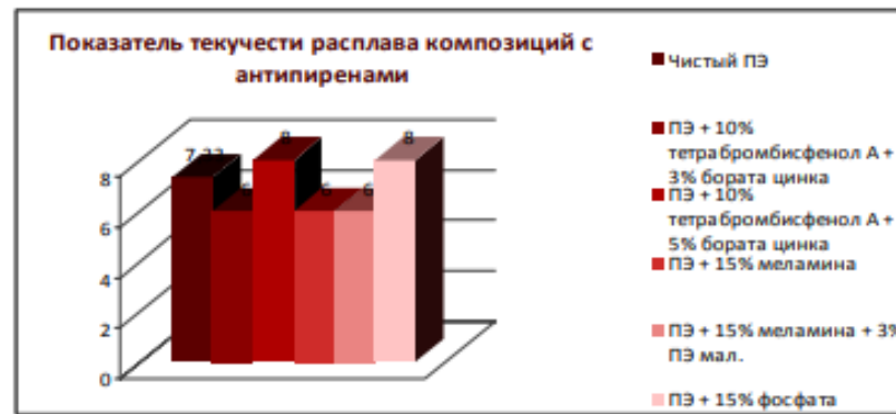
Fig.3. Diagram of MFI values depending on the content of flame retardants in the composition
